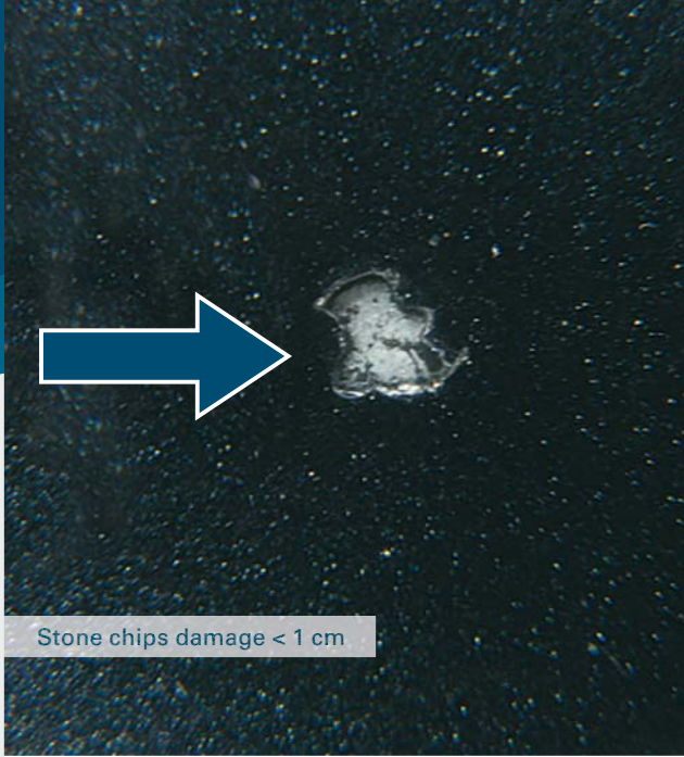
Small scratch, can be polished away < 1 cm
